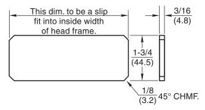
To locate end plates (by others) on hollow metal mounting channel first determine hand of door. Then, holding mounting channel in front of you with end stamped HINGE away from you, locate end plates as shown. THE BOTTOM EDGES OF THE END PLATES AND THE MOUNTING CHANNEL MUST BE FLUSH.
