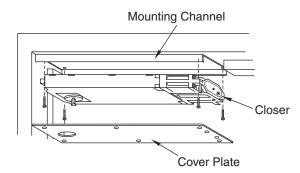
4. Slide assembled unit (with end plates welded to mounting channel) into head jamb. Important: End of channel stamped HINGE must face hinge jamb of frame. Assembly should be clamped down flush with the inside of the head frame.
