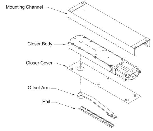
Mounting Channel Prep: Make (2) reinforcement end plates for Mounting Channel.
