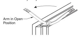
b. Remove arm from spindle.
