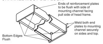
Clamp end plates to mounting channel. Tack weld end plates to mounting channel. Side legs of mounting channel must be at right angles to top of channel and parallel to one another after end plates are welded in place.
