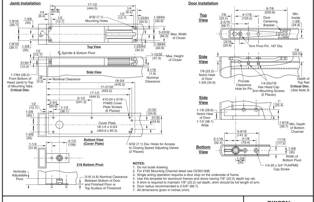
M700 Single Acting & M800 Double Acting Overhead Concealed Door Closer Center Hung for Metal Doors and Frames ASSA ABLOY
