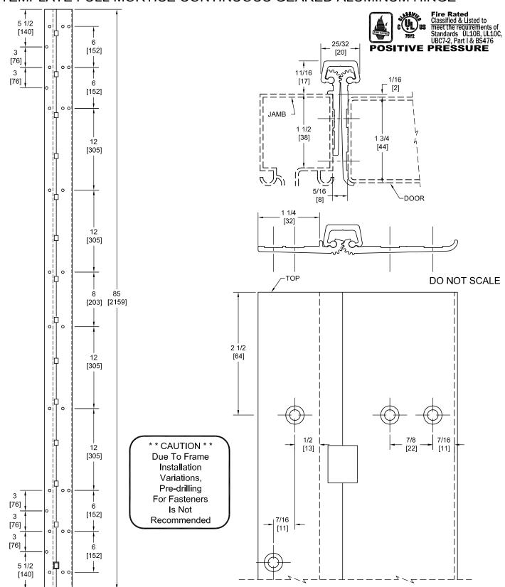
PEMKO Template Full Mortise Continuous Geared Aluminum Hinges CSPFM85/DSPFM85 are made to conform to this drawing. PEMKO CSPFM85/DSPFM85 hinges can be supplied with Electric Functions - See Electrical Application Section. Machine Screw Size - No. 12-24 x 7/16 FHUC Thread-forming.
