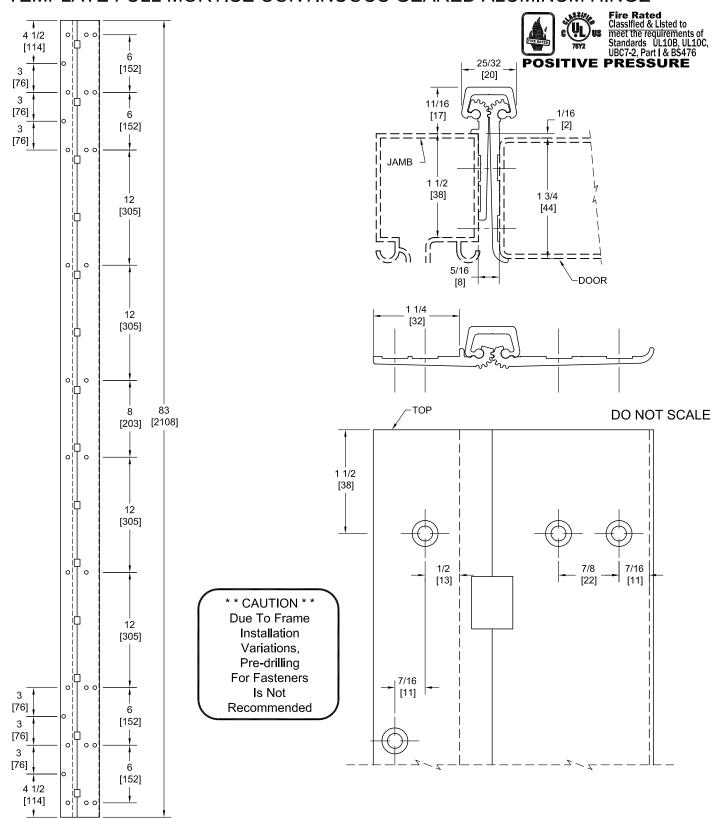
PEMKO Template Full Mortise Continuous Geared Aluminum Hinges CSPFM83/DSPFM83 are made to conform to this drawing. PEMKO CSPFM83/DSPFM83 hinges can be supplied with Electric Functions - See Electrical Application Section. Machine Screw Size - No. 12-24 x 7/16 FHUC Thread-forming.
