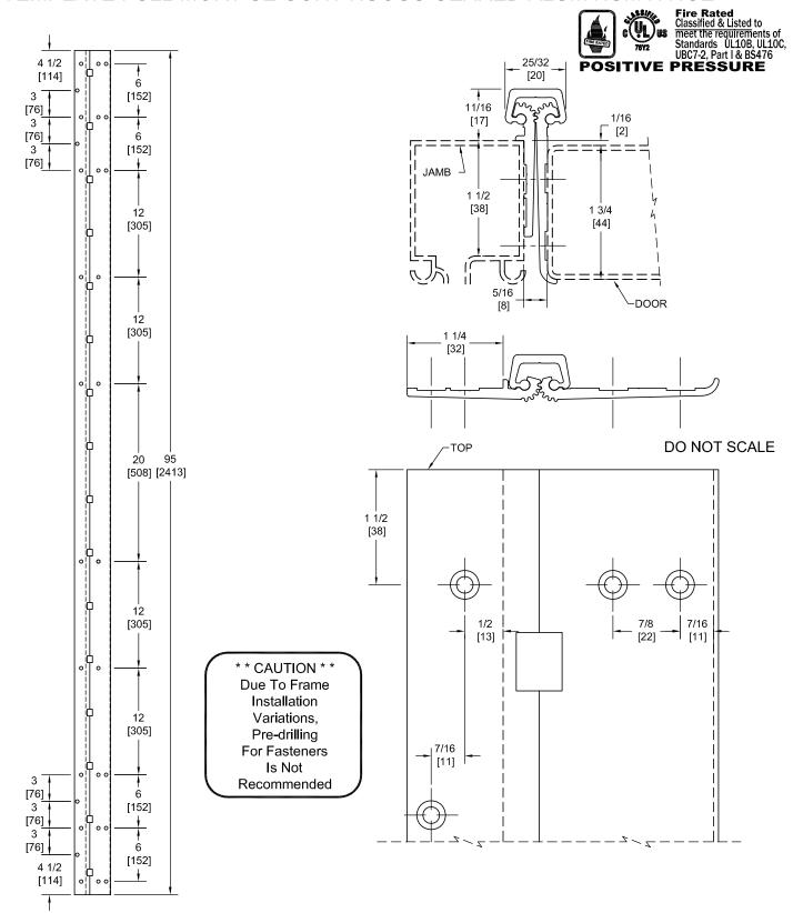
PEMKO Template Full Mortise Continuous Geared Aluminum Hinges CSPFM95/DSPFM95 are made to conform to this drawing. PEMKO CSPFM95/DSPFM95 hinges can be supplied with Electric Functions - See Electrical Application Section. Machine Screw Size - No. 12-24 x 7/16 FHUC Thread-forming.
