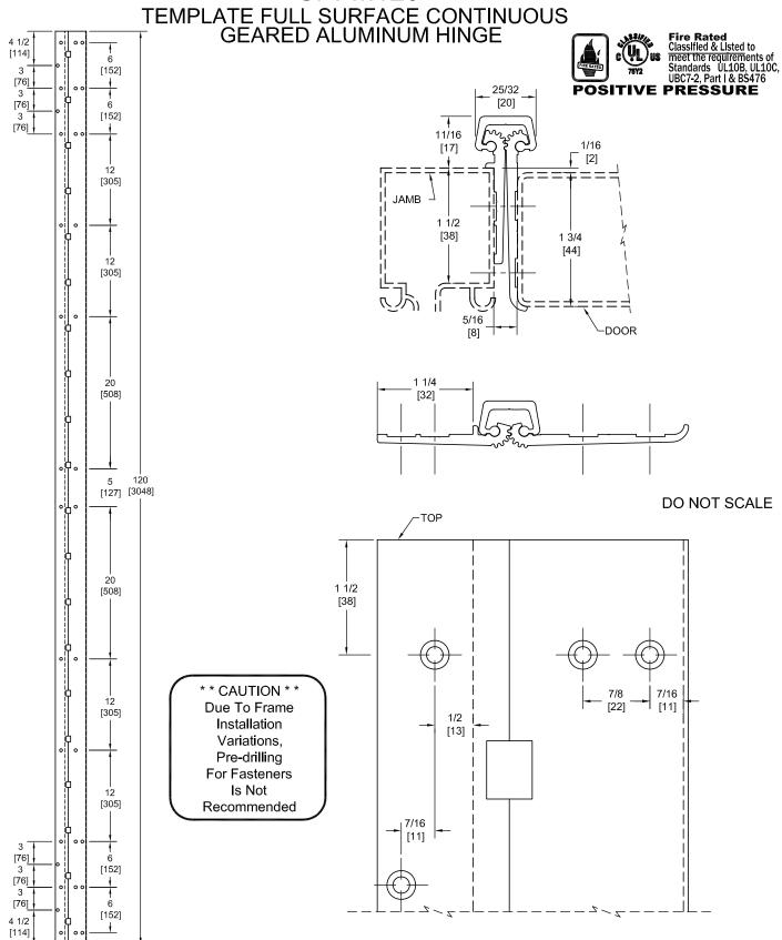
PEMKO Template Full Mortise Continuous Geared Aluminum Hinges CSPFM120/DSPFM120 are made to conform to this drawing. PEMKO CSPFM120/DSPFM120 hinges can be supplied with Electric Functions - See Electrical Application Section. Machine Screw Size - No. 12-24 x 7/16 FHUC Thread-forming.
