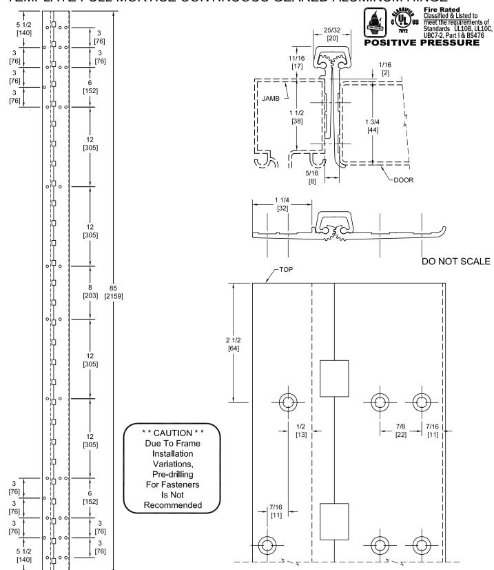
PEMKO Template Full Mortise Continuous Geared Aluminum Hinges CSPFM85-HD/DSPFM85-HD are made to conform to this drawing. PEMKO CSPFM85-HD/DSPFM85-HD hinges can be supplied with Electric Functions - See Electrical Application Section. Machine Screw Size - No. 12-24 x 7/16 FHUC Thread-forming.
