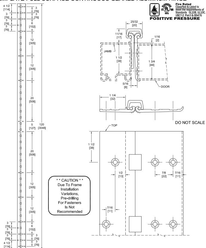
PEMKO Template Full Mortise Continuous Geared Aluminum Hinges CSPFM120-HD/DSPFM120-HD are made to conform to this drawing. PEMKO CSPFM120-HD/DSPFM120-HD hinges can be supplied with Electric Functions - See Electrical Application Section.
