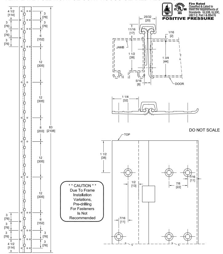
PEMKO Template Full Mortise Continuous Geared Aluminum Hinges CSPFM83-HD/DSPFM83-HD are made to conform to this drawing. PEMKO CSPFM83-HD/DSPFM83-HD hinges can be supplied with Electric Functions - See Electrical Application Section. Machine Screw Size - No. 12-24 x 7/16 FHUC Thread-forming.
