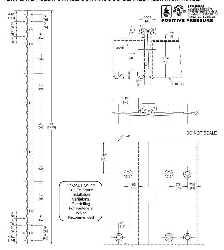
PEMKO Template Full Mortise Continuous Geared Aluminum Hinges CSPFM95-HD/DSPFM95-HD are made to conform to this drawing. PEMKO CSPFM95-HD/DSPFM95-HD hinges can be supplied with Electric Functions - See Electrical Application Section. Machine Screw Size - No. 12-24 x 7/16 FHUC Thread-forming.
