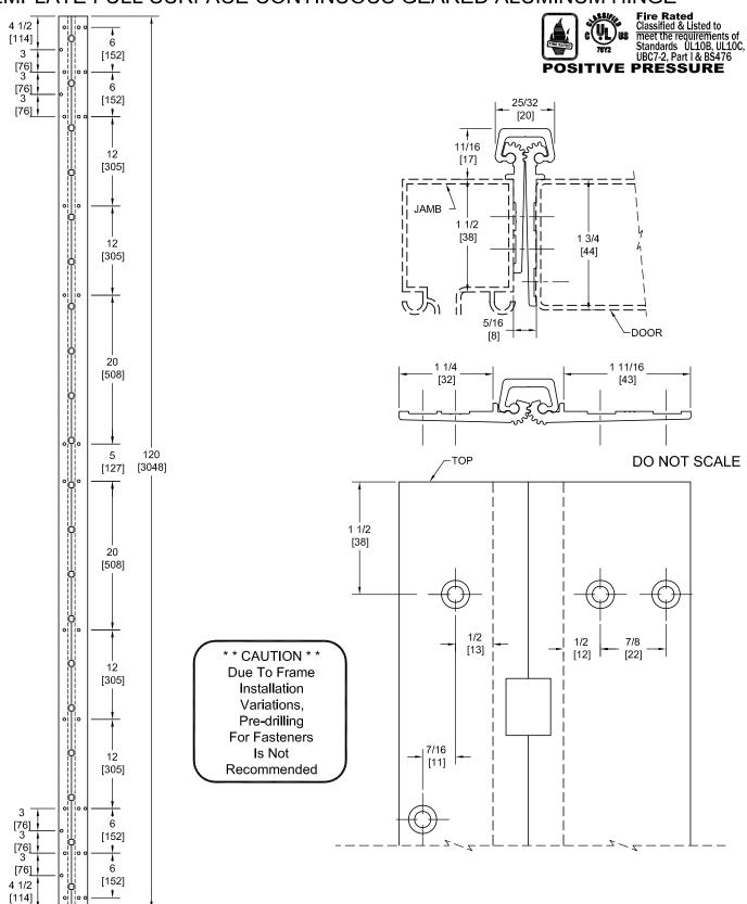
PEMKO Template Full Mortise Continuous Geared Aluminum Hinges CSPFM120SLF/DSPFM120SLF are made to conform to this drawing. PEMKO CSPFM120SLF/DSPFM120SLF hinges can be supplied with Electric Functions - See Electrical Application Section. Machine Screw Size - No. 12-24 x 7/16 FHUC Thread-forming.
