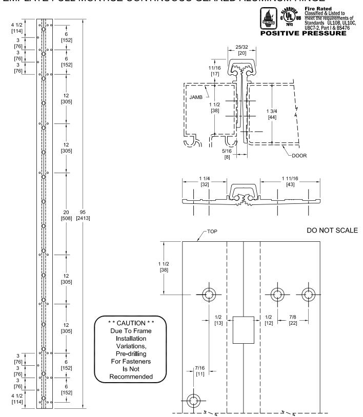
PEMKO Template Full Mortise Continuous Geared Aluminum Hinges CSPFM95SLF/DSPFM95SLF are made to conform to this drawing. PEMKO CSPFM95SLF/DSPFM95SLF hinges can be supplied with Electric Functions - See Electrical Application Section. Machine Screw Size - No. 12-24 x 7/16 FHUC Thread-forming.
