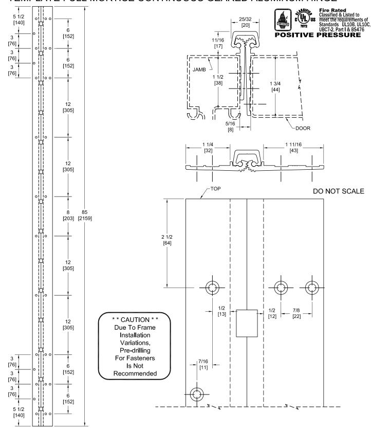
PEMKO Template Full Mortise Continuous Geared Aluminum Hinges CSPFM8\SSLF/DSPFM85SLF are made to conform to this drawing. PEMKO CSPFM85SLF/DSPFM85SLF hinges can be supplied with Electric Functions - See Electrical Application Section. Machine Screw Size - No. 12-24 x 7/16 FHUC Thread-forming.
