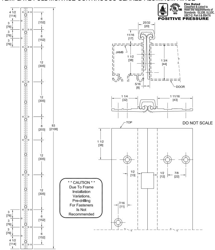
PEMKO Template Full Mortise Continuous Geared Aluminum Hinges CSPFM83SLF/DSPFM83SLF are made to conform to this drawing. PEMKO CSPFM83SLF/DSPFM83SLF hinges can be supplied with Electric Functions - See Electrical Application Section. Machine Screw Size - No. 12-24 x 7/16 FHUC Thread-forming.
