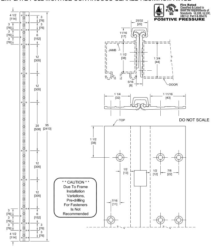
PEMKO Template Full Mortise Continuous Geared Aluminum Hinges CSPFM95SLF-HD/DSPFM95SLF-HD are made to conform to this drawing. PEMKO CSPFM95SLF-HD/DSPFM95SLF-HD hinges can be supplied with Electric Functions - See Electrical Application Section. Machine Screw Size - No. 12-24 x 7/16 FHUC Thread-forming.
