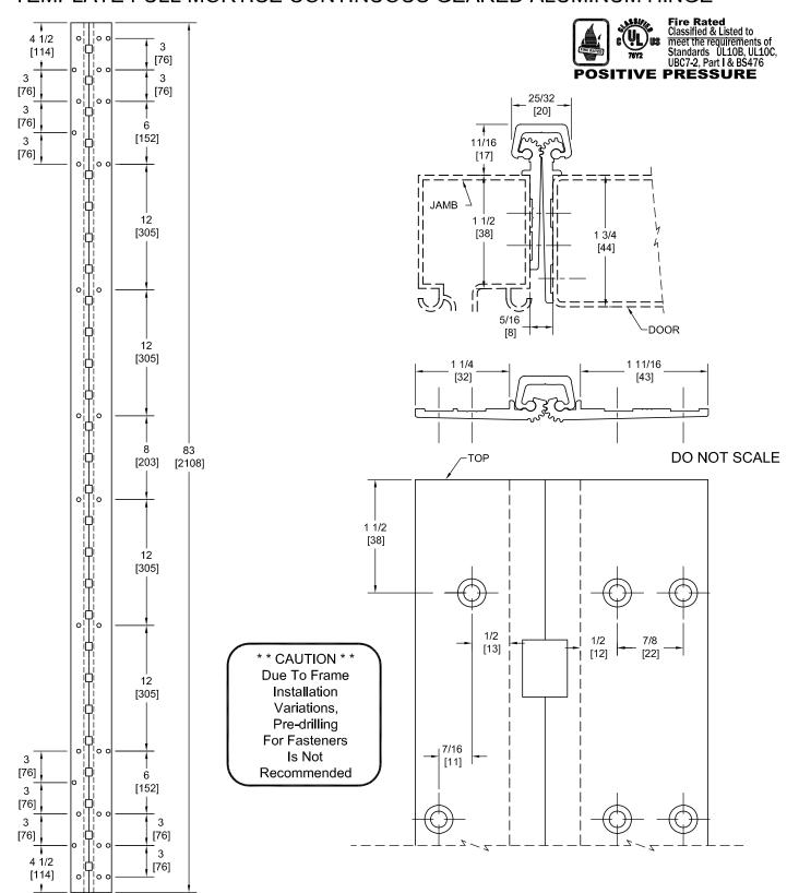
PEMKO Template Full Mortise Continuous Geared Aluminum Hinges CSPFM83SLF-HD/DSPFM83SLF-HD are made to conform to this drawing. PEMKO CSPFM83SLF-HD/DSPFM83SLF-HD hinges can be supplied with Electric Functions - See Electrical Application Section. Machine Screw Size - No. 12-24 x 7/16 FHUC Thread-forming.
