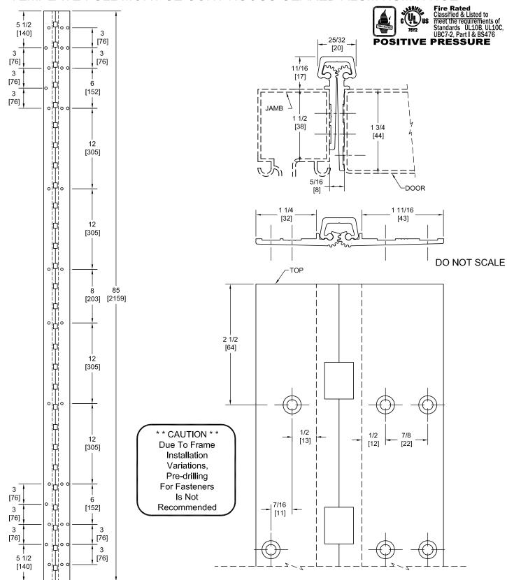
PEMKO Template Full Mortise Continuous Geared Aluminum Hinges CSPFM85SLF-HD/DSPFM85SLF-HD are made to conform to this drawing. PEMKO CSPFM85SLF-HD/DSPFM85SLF-HD hinges can be supplied with Electric Functions - See Electrical Application Section. Machine Screw Size - No. 12-24 x 7/16 FHUC Thread-forming.
