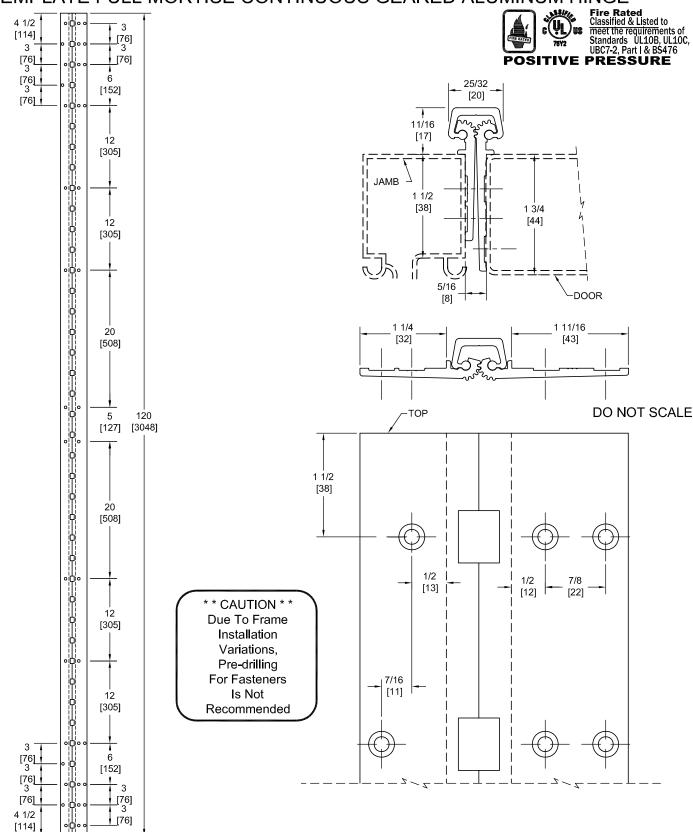
PEMKO Template Full Mortise Continuous Geared Aluminum Hinges CSPFM120SLF-HD/DSPFM120SLF-HD are made to conform to this drawing. PEMKO CSPFM120SLF-HD/DSPFM120SLF-HD hinges can be supplied with Electric Functions - See Electrical Application Section. Machine Screw Size - No. 12-24 x 7/16 FHUC Thread-forming.
