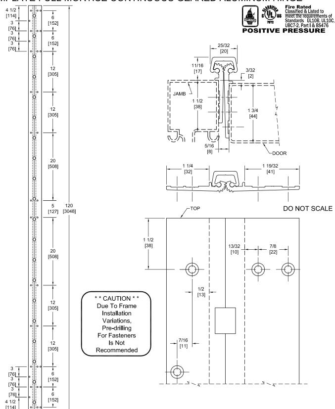
PEMKO Template Full Mortise Continuous Geared Aluminum Hinges CSPFM120SLI/DSPFM120SLI are made to conform to this drawing. PEMKO CSPFM120SLI/DSPFM120SLI hinges can be supplied with Electric Functions - See Electrical Application Section. Machine Screw Size - No. 12-24 x 7/16 FHUC Thread-forming.
