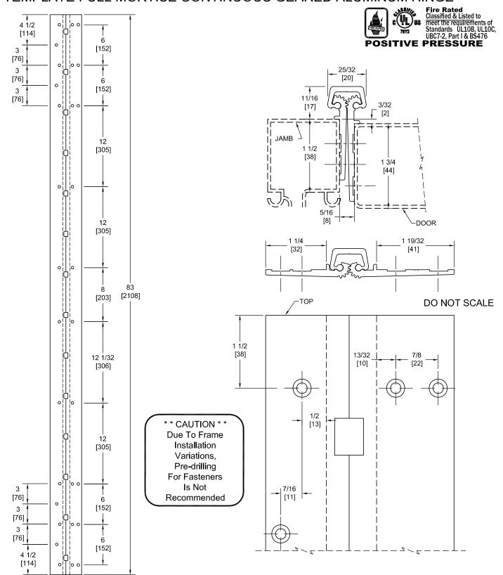
PEMKO Template Full Mortise Continuous Geared Aluminum Hinges CSPFM83SLI/DSPFM83SLI are made to conform to this drawing. PEMKO CSPFM83SLI/DSPFM83SLI hinges can be supplied with Electric Functions - See Electrical Application Section. Machine Screw Size - No. 12-24 x 7/16 FHUC Thread-forming.
