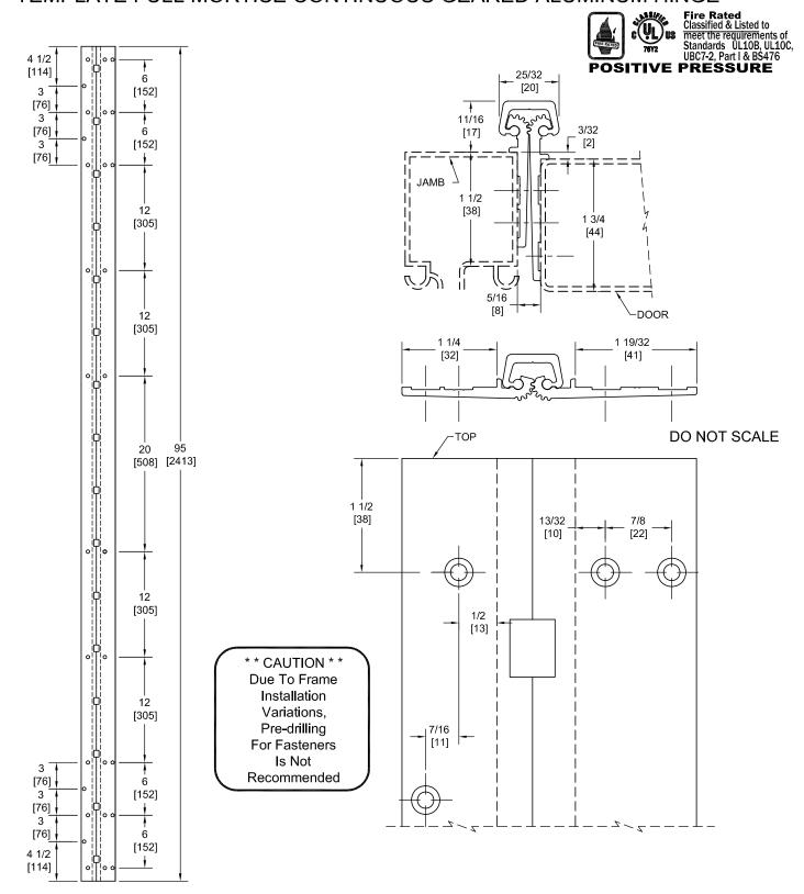
PEMKO Template Full Mortise Continuous Geared Aluminum Hinges CSPFM95SLI/DSPFM95SLI are made to conform to this drawing. PEMKO CSPFM95SLI/DSPFM95SLI hinges can be supplied with Electric Functions - See Electrical Application Section. Machine Screw Size - No. 12-24 x 7/16 FHUC Thread-forming.
