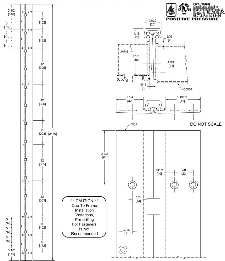
PEMKO Template Full Mortise Continuous Geared Aluminum Hinges CSPFM85SLI/DSPFM85SLI are made to conform to this drawing. PEMKO CSPFM85SLI/DSPFM85SLI hinges can be supplied with Electric Functions - See Electrical Application Section. Machine Screw Size - No. 12-24 x 7/16 FHUC Thread-forming.
