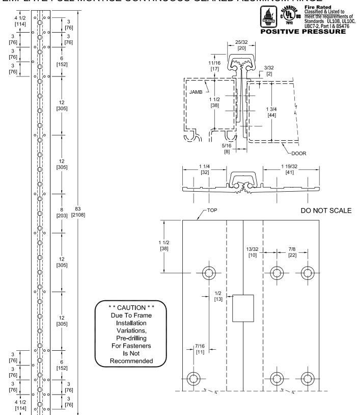
PEMKO Template Full Mortise Continuous Geared Aluminum Hinges CSPFM83SLI-HD/DSPFM83SLI-HD are made to conform to this drawing. PEMKO CSPFM83SLI-HD/DSPFM83SLI-HD hinges can be supplied with Electric Functions - See Electrical Application Section. Machine Screw Size - No. 12-24 x 7/16 FHUC Thread-forming.
