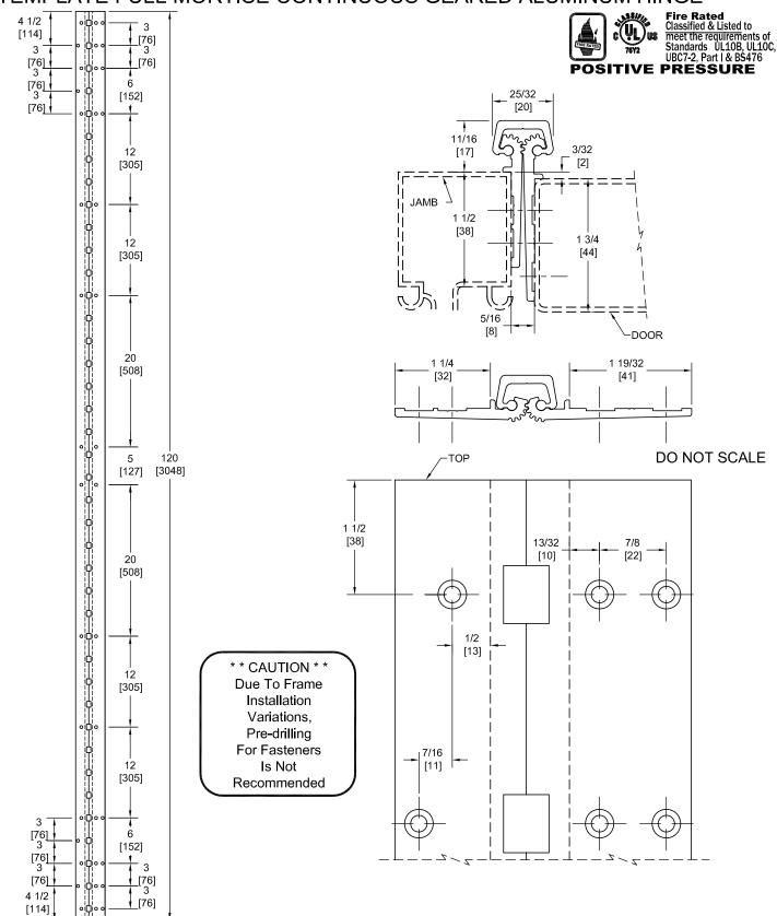
PEMKO Template Full Mortise Continuous Geared Aluminum Hinges CSPFM120SLIHD/DSPFM120SLIHD are made to conform to this drawing. PEMKO CSPFM120SLIHD/DSPFM120SLIHD hinges can be supplied with Electric Functions - See Electrical Application Section. Machine Screw Size - No. 12-24 x 7/16 FHUC Thread-forming.
