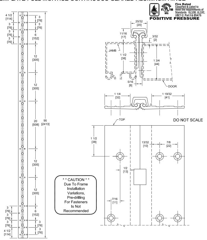
PEMKO Template Full Mortise Continuous Geared Aluminum Hinges CSPFM95SLI-HD/DSPFM95SLI-HD are made to conform to this drawing. PEMKO CSPFM95SLI-HD/DSPFM95SLI-HD hinges can be supplied with Electric Functions - See Electrical Application Section. Machine Screw Size - No. 12-24 x 7/16 FHUC Thread-forming.
