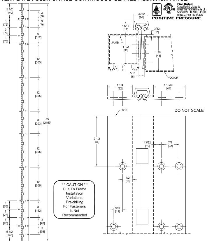
PEMKO Template Full Mortise Continuous Geared Aluminum Hinges CSPFM85SLI-HD/DSPFM85SLI-HD are made to conform to this drawing. PEMKO CSPFM85SLI-HD/DSPFM85SLI-HD hinges can be supplied with Electric Functions - See Electrical Application Section. Machine Screw Size - No. 12-24 x 7/16 FHUC Thread-forming.
