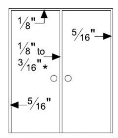
\* Certain door and frame conditions may require an extra 1/32"-1/16" clearance. Excessive clearance on fire rated assemblies may violate the requirements of NFPA 80.
