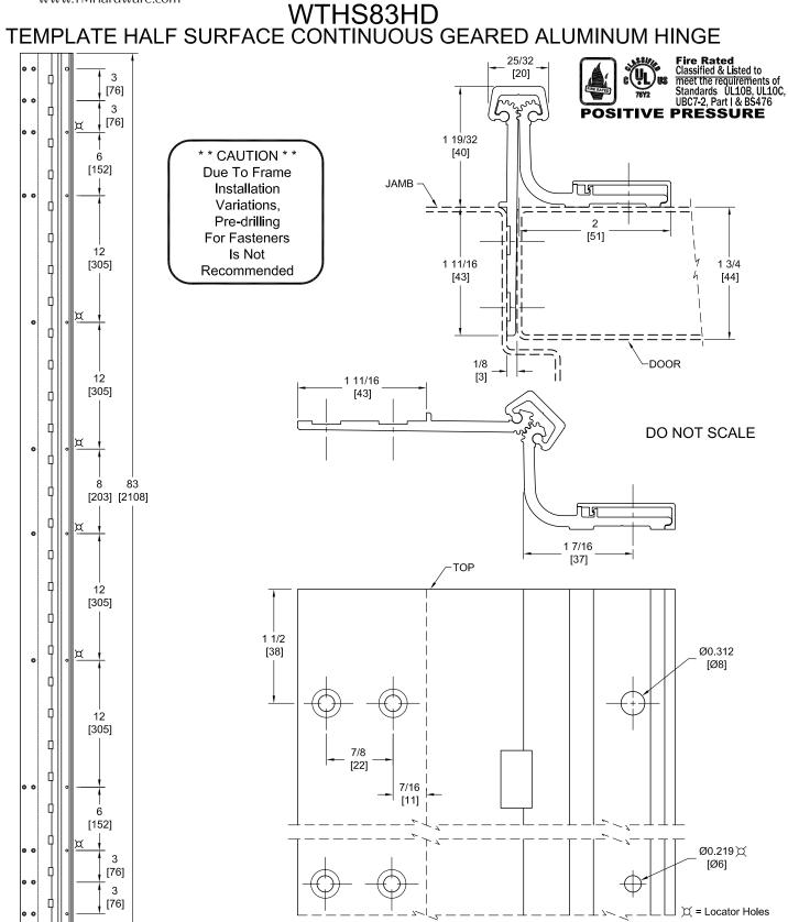
PEMKO Template Full Surface Continuous Geared Aluminum Hinges CWTHS83HD/DWTHS83HD are made to conform to this drawing. Machine Screw Size - Jamb Leaf - No. 12-24 x 7/16 FHUC Thread-forming.
