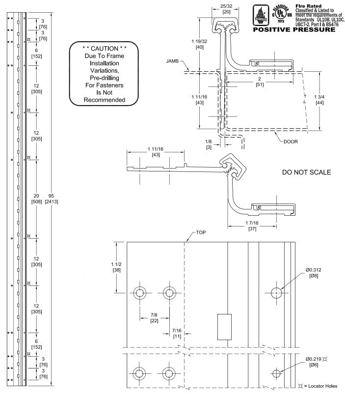
PEMKO Template Full Surface Continuous Geared Aluminum Hinges CWTHS95HD/DWTHS95HD are made to conform to this drawing. Machine Screw Size - Jamb Leaf - No. 12-24 x 7/16 FHUC Thread-forming.
