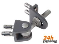
180° hinge that can quickly be mounted without any welding being required. It also offers all advantages of the GBMU4D range: vandal-proof, adjustment of height, depth and distance between gate and post; and left/right interchangeable so it can be used for both left and right handed gates. BOLTON4D is available in M12 and M16, and always in 2 versions: one with Quick-Fix on both sides and one with Quick-Fix on the post, and on gate side a bolt through fixing for gate frames from 1.6" to 2.4".
