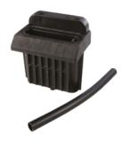
Strong ground stop and receiver for double leaf gates. It is recommended to be used in combination with the internal drop bolt SUBY. "Centered" refers to the positioning of the receiving ground pot, which is "centered" under the gate leaf when the gate is closed. The CGS has a removable receiver for easy and fast cleaning of the ground pot.
