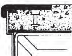
Type 101SP with concealed integral anchor in steel pan stair.
