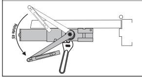
Use adjustable wrench to rotate spindle 45° counterclockwise for Right Hand Door or clockwise for Left Hand Door. Place main arm on spindle so that it is 45° or less from the tube end of the closer body. Secure main arm and spindle by tightening spindle bolt.
