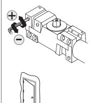
Adjust latch speed so door completely closes and latches.
