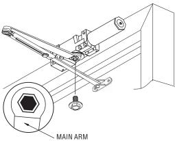
Orient main arm  $90^\circ$  from the closer body. Press arm down on spindle and secure with spindle bolt.
