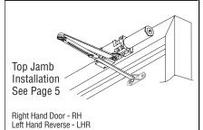
• These door closers should **NOT** be installed on the exposed side (weather side) of exterior doors.
