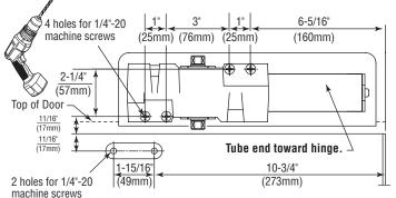
An optional mounting plate is required where the head frame face is less than 3-1/2" (89mm). Plate requires 1-3/4" (44mm) minimum head frame.
