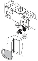
Adjust backcheck accordingly to prevent excessive opening speed.
