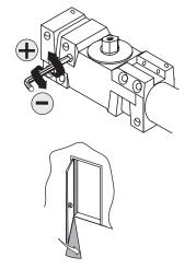
Adjust delay action accordingly to obtain desired delay time.
