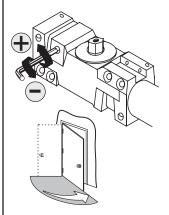
Note: Adjust closing time speed to between 3 and 7 seconds from 90 to 0. Greater closing times may be required for elderly or handicapped.
