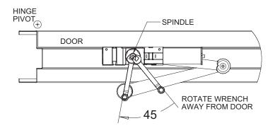
Use an adjustable wrench to rotate the bottom pinion shaft about 45 degrees in the direction away from the door.
