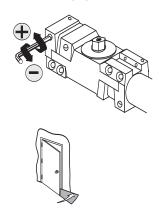
Adjust latch speed so door completely closes and latches
