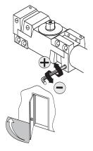
Adjust backcheck accordingly to prevent excessive opening speed.
