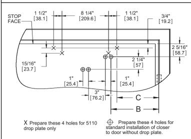
Note: Drop plate works with a minimum top rail of 2 1/2".
