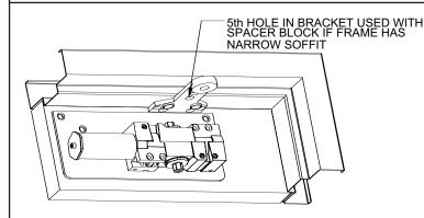
If using a drop plate, screw the drop plate to the door using 1/4-20 screws. Screw closer to the drop plate using 7/16" long machine screws.
