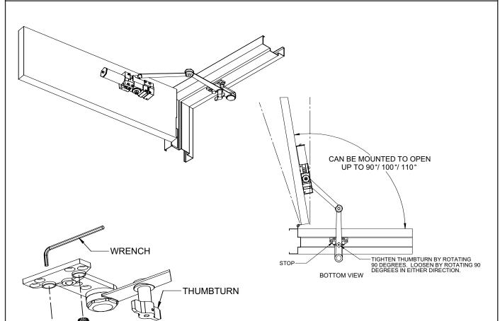
Removable stop can be used for right hand or left hand application (currently shown in right hand application). Stop can only be removed when arm is not attached to the frame. Use a hex wrench to unscrew stop and move it. See picture to the left. To engage hold open feature, open door to the stop and rotate thumbturn 90 degrees. To release, rotate thumbturn 90 degree in either direction.
