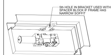
Before mounting closers, make sure selector valve (found on back of closer) is screwed in.
