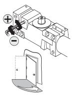
Note: Adjust closing time speed between 3 and 7 seconds from 90° to 0°. Greater closing times may be required for elderly or handicapped.
