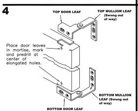
To allow for vertical adjustment and sufficient clearance under the door, the bottom mullion leaf should be mounted at least 1/4" off the floor. If carpet or other special floor coverings are used, additional clearance should be allowed equal to their thickness.
