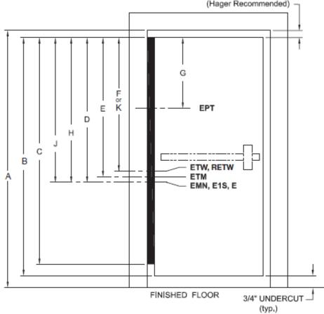
For ease of ordering, Hager Companies has established standard locations for power transfer cutouts. All standard location dimensions are referenced from the top edge of the door to the centerline of the power transfer cutout. Please specify handing.
