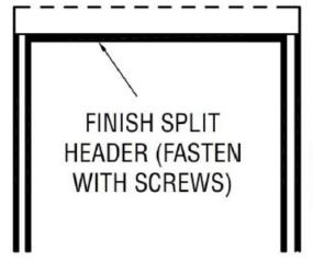
Install finish split header to the exposed wood on either side of the track. To allow for future door adjustment or removal, at least one finished split header should be attached with screws only; the one on your right hand overhead as you face the door in the pocket is recommended.
