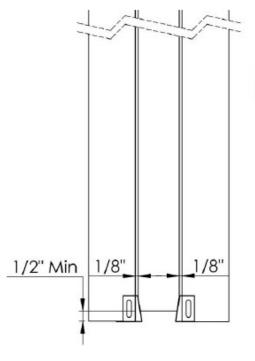
Install Door guides to finish split jamb and adjust to within 1/16" of door on either side
