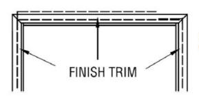
Install finish trim or casing. Fasten finish header trim to EITHER header OR wall, NOT BOTH, so the header can be remover later without damage.
