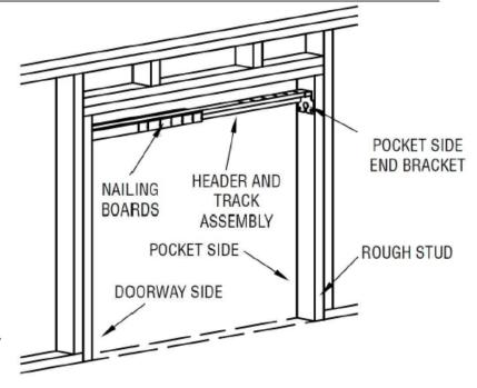
Check the door thickness. When installed without modifications, this pocket door frame allows 2" (50.8 mm) of free space for the door between the split studs. A 1-3/8" (34.93 mm) door would leave 5/16" (7.94 mm) clearance on each side. A 1-3/4" (44.45 mm) door would leave 1/8" (3.18) clearance on each side.
