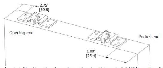
Note: when installing bi-parting doors change Opening distance to 3-3/4" from edge of door.
