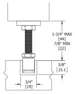
Installation note: Clearance between door bottom and top of 9122 track must be 7/8" (22 mm) minimum to 1-3/4" (44 mm) maximum.
