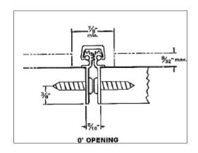
ROTON Model 500- Minimum clearance required between the hinge the edge of the door and the frame is 5/16" (7.9 mm). The maximum allowable trim thickness is 9/32" (7.1 mm) to maintain clearance when the hinge is in its fully open position of 180 degrees.
