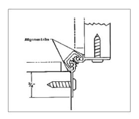
The 500-Series Hinges are supplied in four standard lengths. See chart. If the hinge must be trimmed shorter, determine the desired finished length and mark. Be careful not to cut within 1/2" of a bearing or screw hole. The excess length may be removed all from one end or by cutting equal amounts from both ends.
