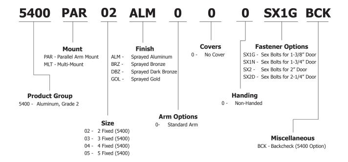
5400 Series closers are sized 2, 3, 4 & 5. Must know size when placing order.
