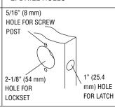
Drill 2-1/8" (54 mm) hole through door face as marked for lockset. (It is recommended that holes be drilled from both sides on wood doors to prevent splitting.) Drill 5/16" (8 mm) holes for screwposts. Drill 1" (25.4 mm) hole in center of door edge for latch.
