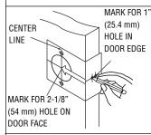
Measure center line of lock; height as desired from finished floor. Select 2-3/4" or optional 2-3/8" backset, fold and apply template to high side of door bevel and mark center of door edge as indicated on template. Mark center hole and screwpost holes on door face through guide on template.
