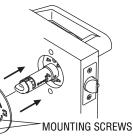
B. Install inside rose liner and align rose liner arrow in the direction of the lock stile. Tighten rose liner to the thru posts using mounting screws.
