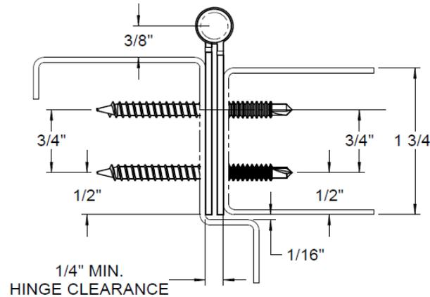
**FIGURE 5: HINGE PLACEMENT & CLEARANCE TEMPLATE**
