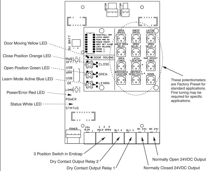
C. Use the supplied green connectors to wire in any devices needing outputs, such as electric strikes, mag locks, exit devices, door open position output, etc. See output definitions below.
