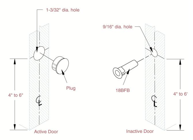
IMPORTANT: The 18BFB will project during a fire. Do not cover with any edge mounted door hardware.
