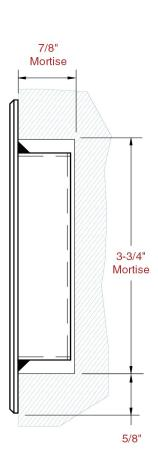
Mortise: 2-7/8"w x 3-3/4"h x 7/8"deep. Drop pull into opening and drill mounting holes using holes in handle as a template.
